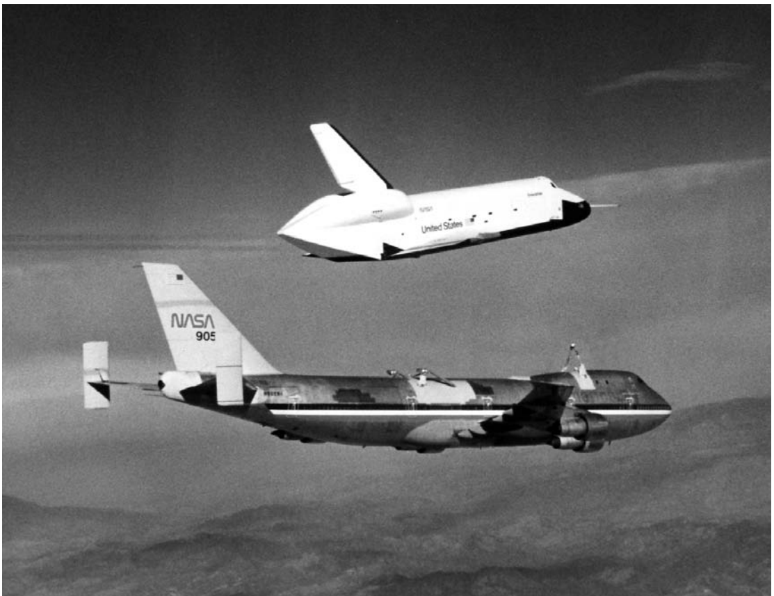
Figure 6. Enterprise free-flight testing after separation from 747. (National Aeronautics and Space Administration, Dryden Aircraft Photo Collection, http://www.dfrc.nasa.gov/Gallery/Photo/ALT/HTML/ECN77-8608.html .)
