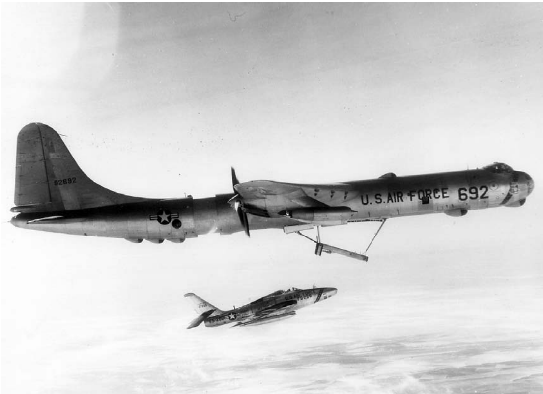
Figure 4. Fighter conveyor. In the early years of the Cold War, the US Air Force needed a reconnaissance aircraft that could reach targets deep in the Soviet Union with the speed and maneuverability to evade Soviet air defenses. The fighter conveyor (FICON) project provided a solution by using the intercontinental RB-36 to carry a jet-powered RF-84 parasite reconnaissance fighter. However, the program was abruptly cancelled in January 1956 when several pilots damaged their airplanes attempting to engage the trapeze. ("Flying Aircraft Carriers of the USAF: Project FICON," Goleta Air and Space Museum , http://www.air-and-space.com/ficon.htm . Dave Menard via Brian Lockett. Reprinted by permission.)
