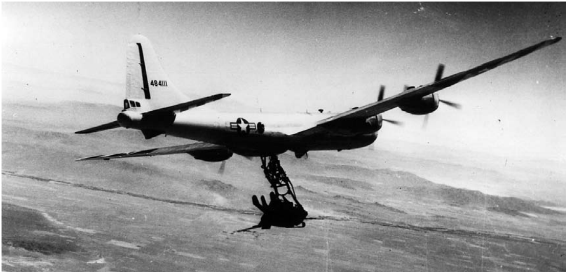
Figure 3. XF-85 Goblin and B-29 mother ship. The McDonnell XF-85 Goblin program sought to provide the B-36 Peacemaker with a fighter for self-defense that the bomber could carry entirely within its bomb bay. An EB-29B replaced the B-36, which was not available for flight-testing. Because of turbulence, only three of seven flights resulted in successful captures. (“Parasite Fighter Programs: Monstro and the XF-85 Goblins,” Goleta Air and Space Museum , http://www.air-and-space.com/goblins.htm . Air Force Flight Test Center History Office via Brian Lockett. Reprinted by permission.)
