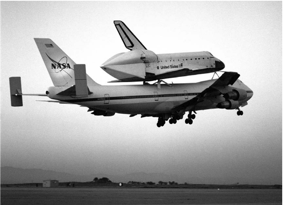
Figure 5. Shuttle carrier aircraft. (National Aeronautics and Space Administration, Dryden Aircraft Photo Collection, http://www.dfrc.nasa.gov/Gallery/Photo/STS-111/HTML/EC02-0131-10.html .)
